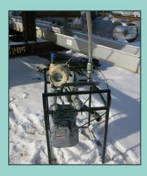
The Hawk 9000 Vent Gas Meter can be used to measure and digitally log low flow vented gas with unparalleled accuracy.
