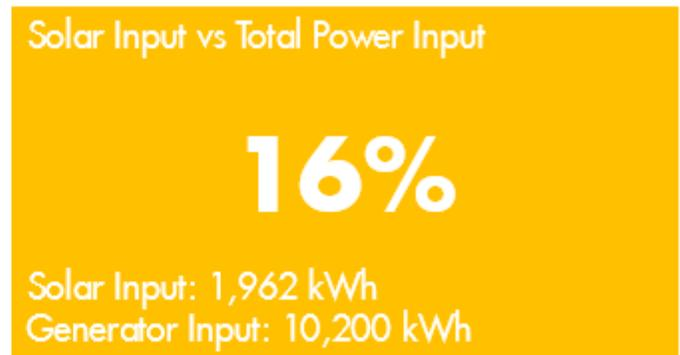
The Shell unit is equipped with remote monitoring and key operating parameters are sent to a server in five-minute intervals. This allows any issues with the unit to be identified and addressed in real-time. For example, the unit shut down on June 15<sup>th</sup>, 2020 due to over-current on the solar charger. Westgen responded within one day to have the breaker replaced and increased the wire gauge as a solution. This change has been incorporated into all EPODs produced moving forward.
