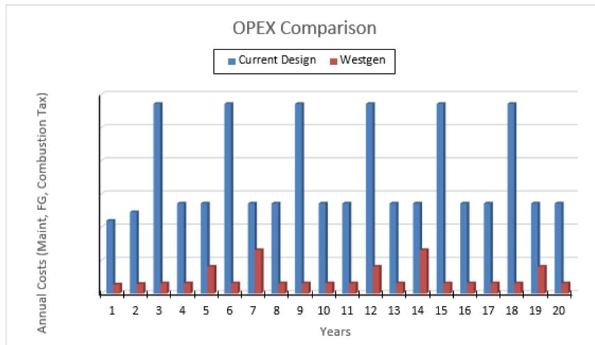
Eliminating the need for a load bank, coupled with the EPOD’s partial duty cycle design and solar power input resulted in reduced fuel gas consumption by \$9,000 per year. The overall reduction in maintenance, fuel gas, and carbon tax resulted in more than 85% savings in operating expenses compared to the previous design.
