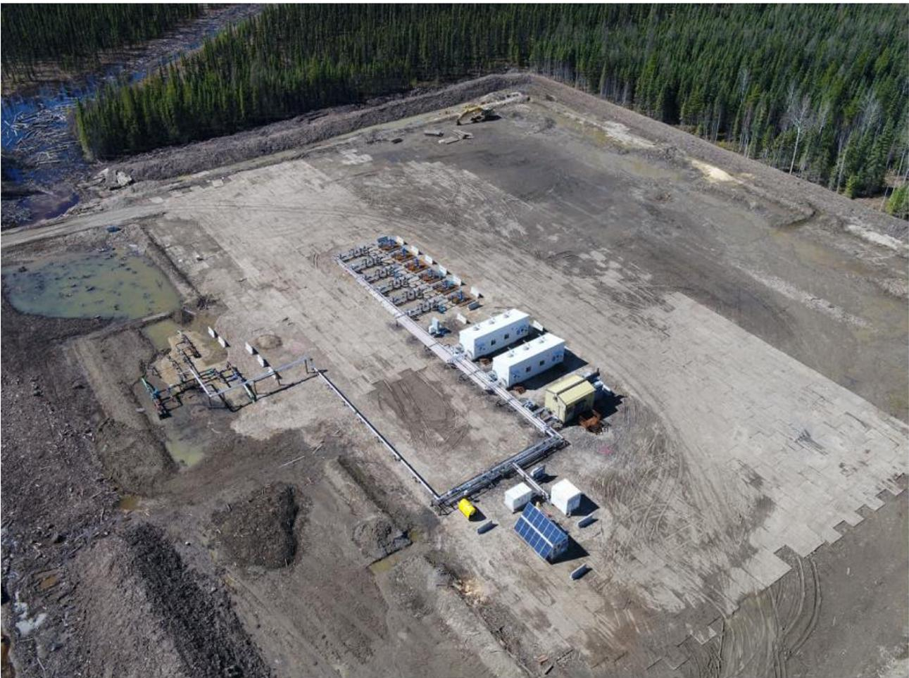
Located in the McKinley / Tony Creek field, near Fox Creek Alberta, the Shell trial wellpad has 6 wells producing from the liquid rich Duvernay shale and uses gas lift for artificial lift.
